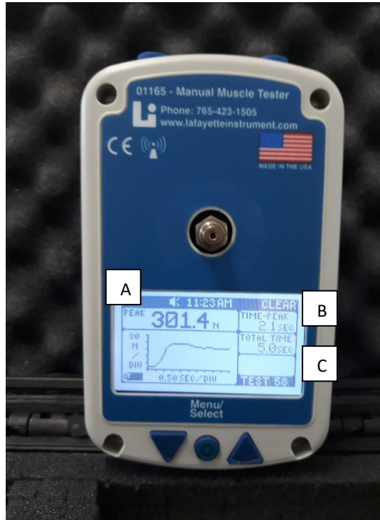
Figure 1 - Lafayette Handheld Dynamometer Testing System Model-01165 - The display shows A: Torque peak, B: Peak time, C: Total test time.
