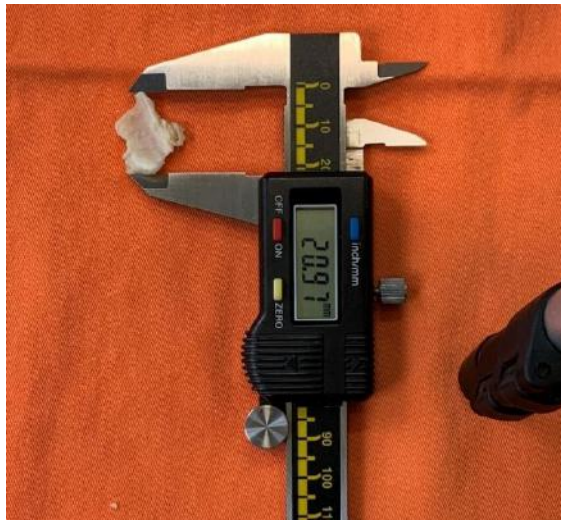
Figure 2 – Disc dimensions evaluation with a digital caliper.
