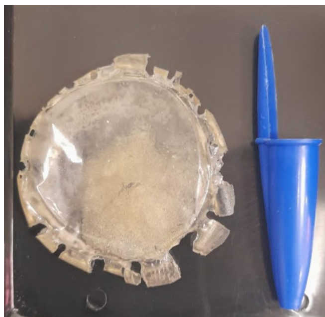
Figure 4 - Film obtained from CBBM24 biomass by casting technique with glycerol plasticizer. *In blue the cap of a pen to reference the size of the film (40 mg of polymer).
